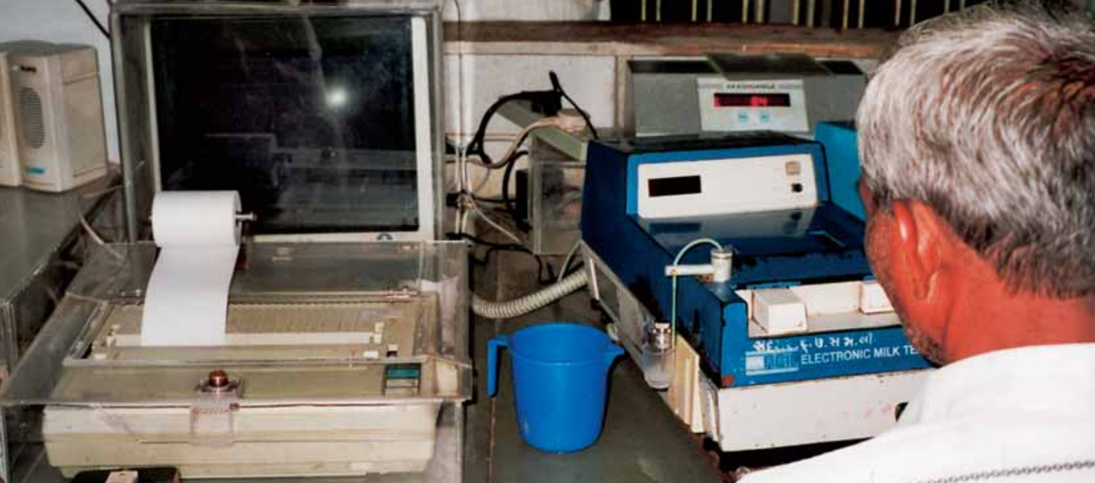
The milk's fat-content is established. Subsequently, the receipt for the milk collection, noting fat content and the total money owed that morning, scrolls out of the printer.
